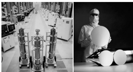
Left: Silicon crystal ingots grown by the Czochralski crystal drawers in the background Right: 200 mm and 300 mm Si
