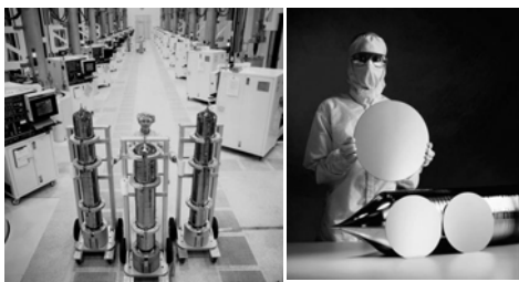
Left: Silicon crystal ingots grown by the Czochralski crystal drawers in the background
