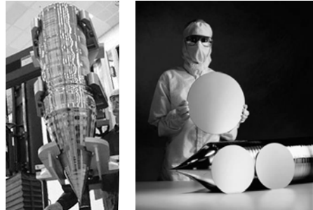
A silicon ingot is a single crystal of Si. Within the bulk of the crystal, the atoms are arranged on a well-defined periodical lattice. The crystal structure is that of diamond.
