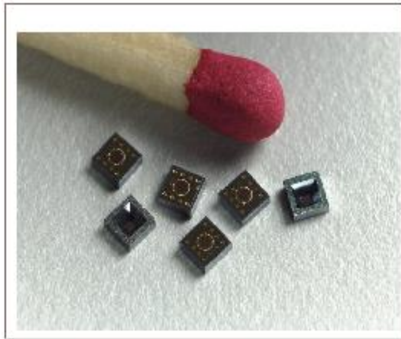
Figure 2. EmKay Sisonic Microphone. This microphone is made from Silicon and is only millimeters large.
