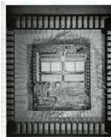
Figure 5-34 Attachment of leads from the Al pads on the periphery of the chip to posts on the package. (Photograph courtesy of Motorola, Inc.)
