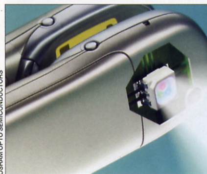
Fig. 1. Applications of white LEDs. Left: a Ford concept car uses Luxeon LEDs from Lumileds as part of an adaptive lighting system that can produce different beam patterns to suit different situations such as highway, in-town or curve driving. Right: white LEDs can replace conventional discharge lamps as the flash for mobile phone cameras. The RGB multichip version can produce a variety of color temperatures.
