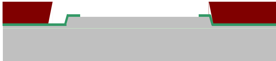
7. Metal Deposition & liftoff
